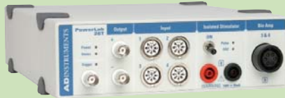
ML4856 PowerLab 26T with human approved dual bio amp, low-voltage and human isolated stimulator, trigger and two to four general-purpose inputs. (Supplied with LabChart and LabTutor)
