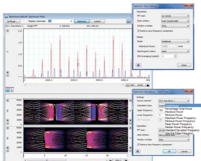
Spectrum View (above), with settings (top right) and calculation options drop down menu (bottom right).
